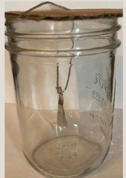
Experimental setup showing how the cardboard, paperclip, and aluminum foil strips should be arranged and placed on the jar.
