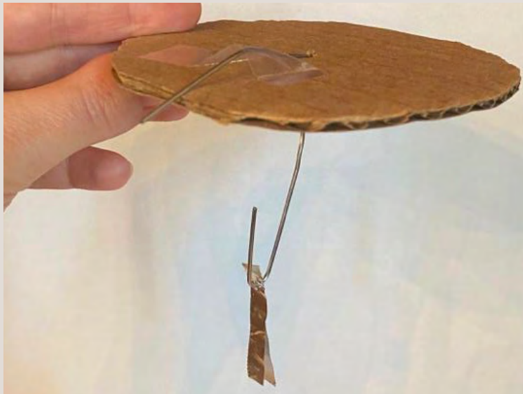
Experimental setup showing how the cardboard, paperclip, and aluminum foil strips should be arranged and placed on the jar.
